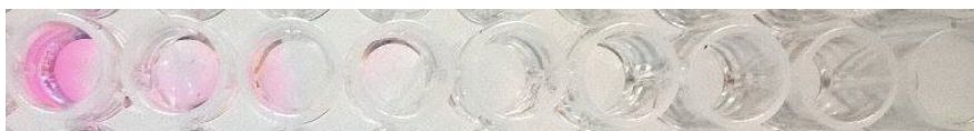
Figure 1. 50 \mu l of Amplex red and HRP was added to 50 \mu l of hydrogen peroxide. From left to right the concentration of hydrogen peroxide was 2.5 \mu M, 1.25 \mu M, 0.62 \mu M, 0.31 \mu M, 0.15 \mu M respectively. The minimum limit of detection was determined as 0.31 \mu M.
