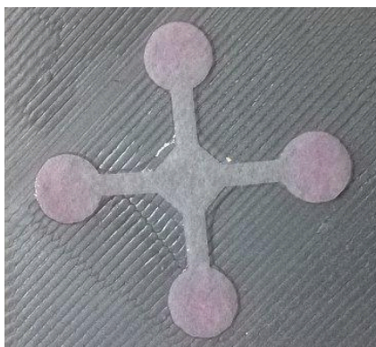
Figure 2. A demonstration of the biosensor sensing 10 \mu M of H 2 O 2 with Horseradish peroxidase and amplex red on the bioactive zones. 20 \mu l of the hydrogen peroxide containing solution was added to the application zone. Time to detection was 3 minutes.
