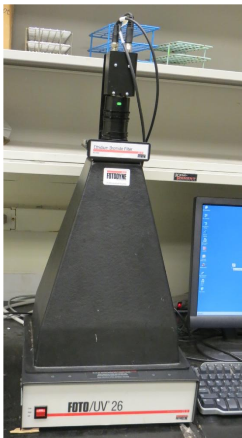
Figure 29 – G7A Transilluminator with digital camera system
