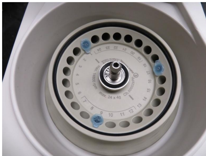
Figure 16 – A balanced rotor in which tubes of the same volume are spaced evenly around the rotor.
