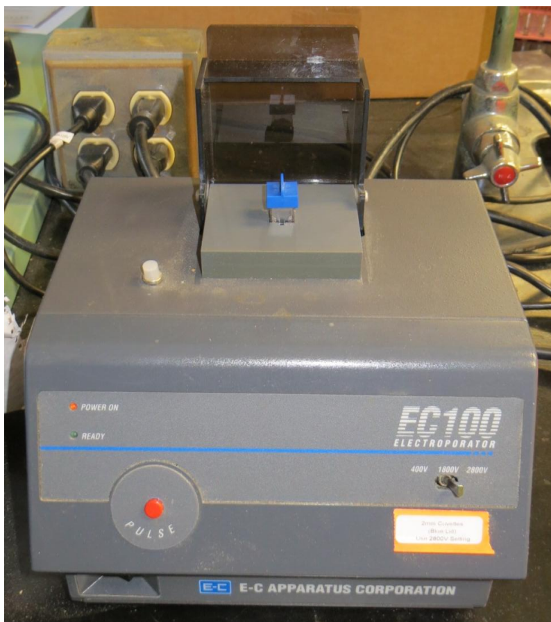
Figure 23 – iGEM lab electroporator with cuvette
