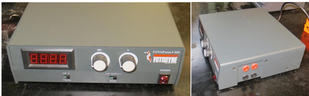
Figure 24 – iGEM gel electrophoresis power supply
