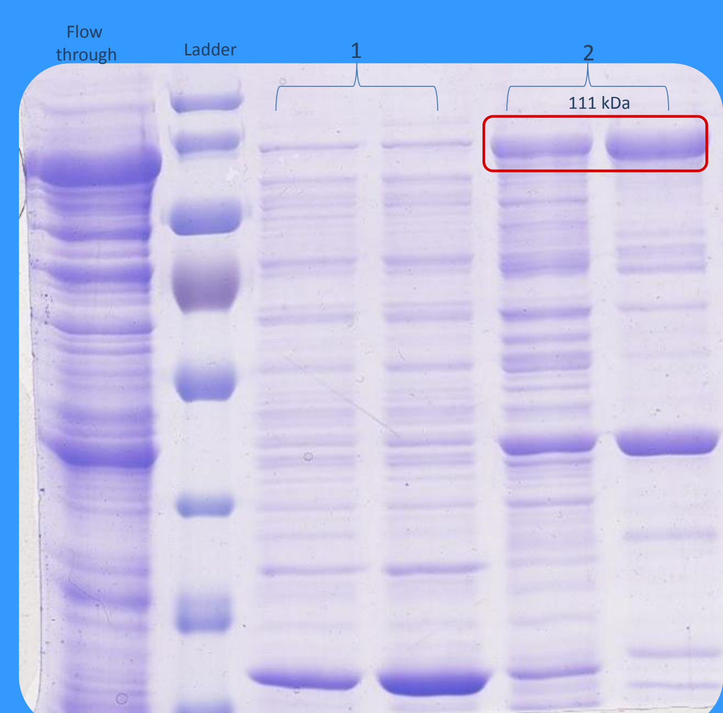
A) SDS gel of the two His-Tag purification peaks. The bands of 111kDa correspond to the scaffoldin
