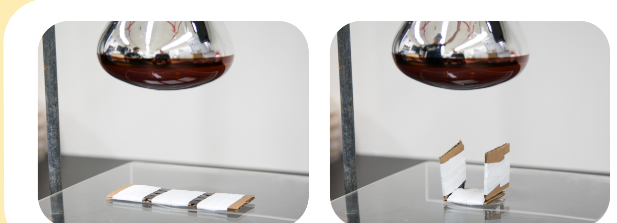
Upon heating, the strips of polystyrene fold at the joints.
